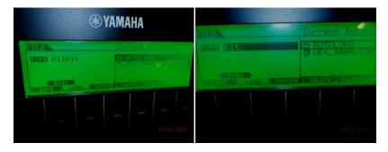
Insert USB Drive into Module (loading a SINGLE KIT) 900 modules
